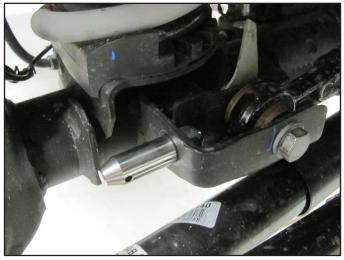
Attach the long mounting post with polyurethane spacer into the factory sway bar link mount. The stud should point towards the center of the vehicle. Tighten the post ensuring the click pin hole is horizontal or parallel with the ground. Tighten to 65 ft-lbs.
