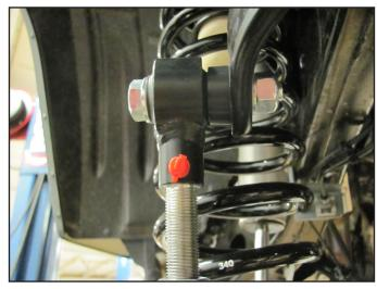
Measure back 1-1/4" from the center of the sway bar link hole or just past the weld at the axle and make a vertical cut line. Cut off the tab at the mark and paint exposed metal.
