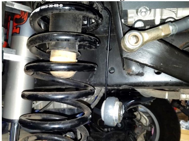
Figure 1. Trackbar End Supported
