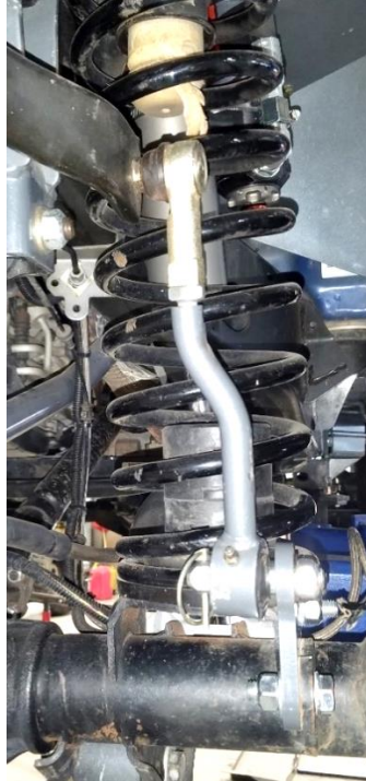
Figures 12. Correctly Installed Driver's Side Sway Bar End Link
