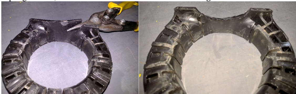
Figures 8 and 9. Trimming Stock Lower Spring Isolator
